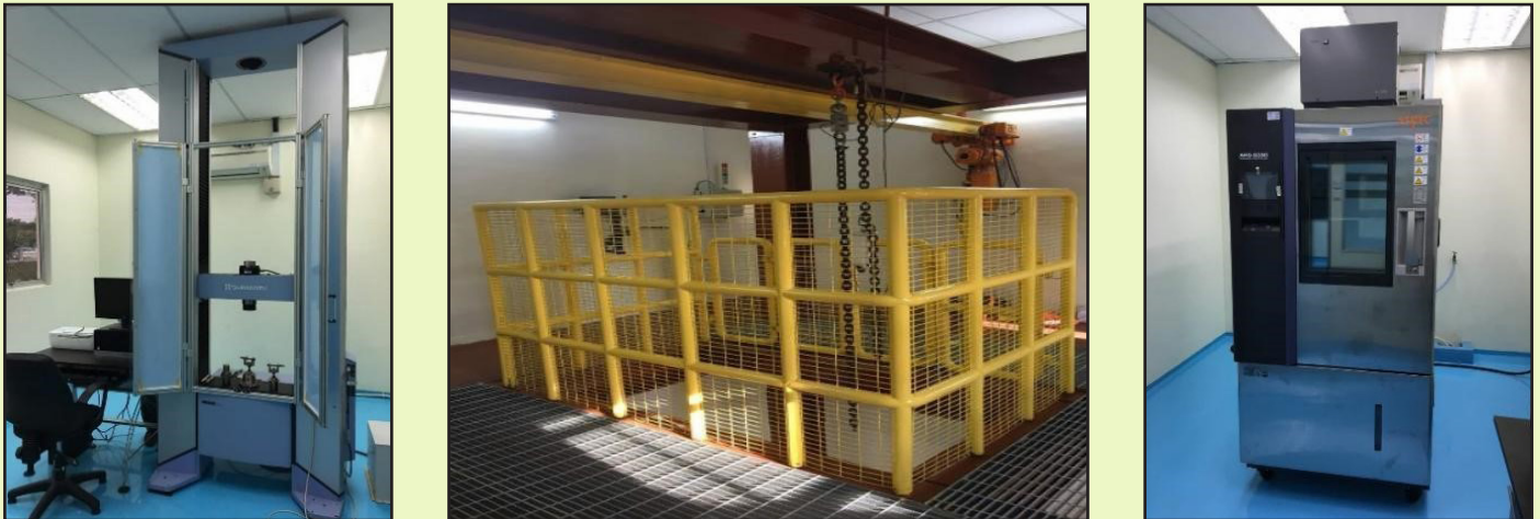
Figure 1.1 Static strength room, dynamic performance tower, and conditioning room
