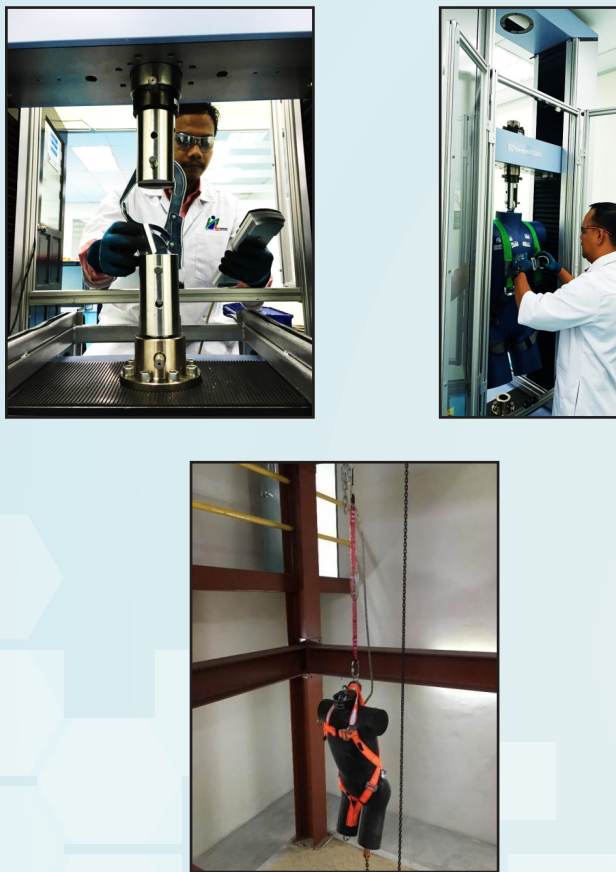
Figure 1.3 1) Static strength test for connector, 2) Static strength test for full body harness, 3) Dynamic performance test for the full body harness
