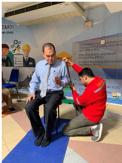
Figure 3 Anthropometer Measurement (Shoulder Elbow Length)
