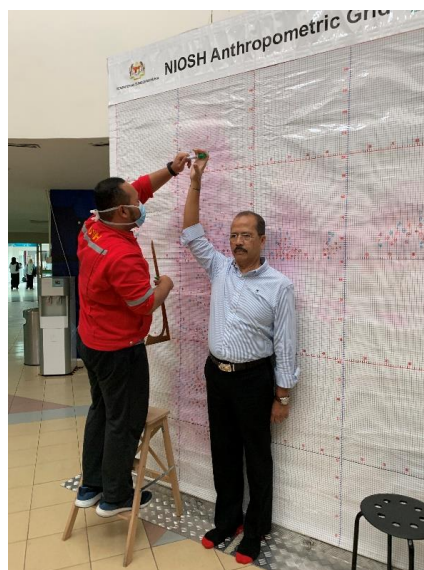
Figure 2 Anthropometric Grid Measurement (Vertical Grip Reach)
