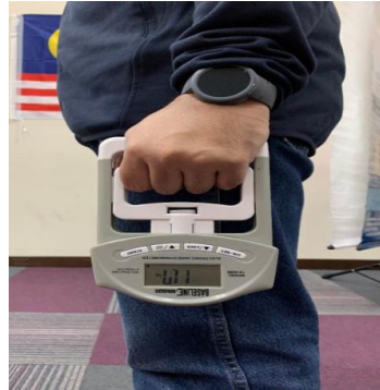
Figure 1 Respondent Gripping the Baseline Digital Smedley Dynamometer during Hand Grip Strength Test
